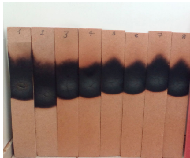
Figure 1. Some burnt MDF specimens after the in-house FR test (treated specimens; 1–2: control; 3–4: Siriono®; 5–6: C7/2; 7–8: C7/3).
