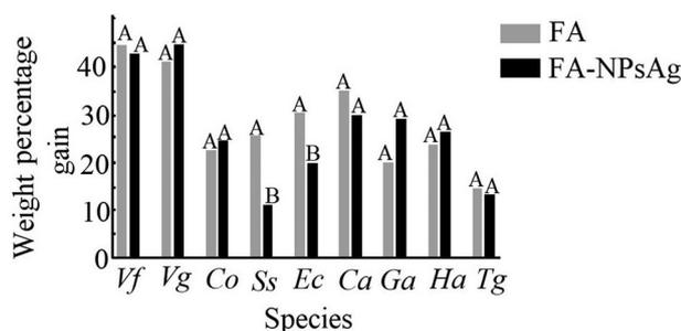
**Figure 1.** Weight percentage gain of wood from nine tropical species of Costa Rica, treated with furfuryl alcohol (FA) and furfuryl alcohol with silver nanoparticles (FA-NPsAg).
