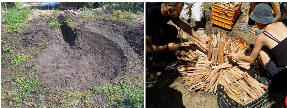
The base pit for tar collection. Left – the pit. The sloped channel will guide the tar into a vessel placed at the lowest point. Right – participants carefully arrange kindling into a circular core, forming the central shaft of a traditional tar mound.
