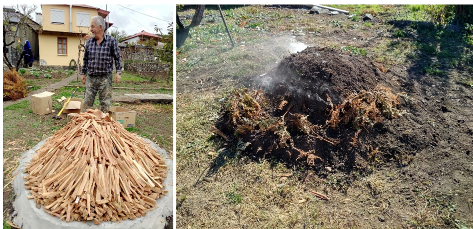
Fig. 4. Traditional tar kiln prepared by stacking split pine wood into a conical mound (left). The tar kiln is covered with soil and ignited (Phot. by K. Paganias, November 2024)
