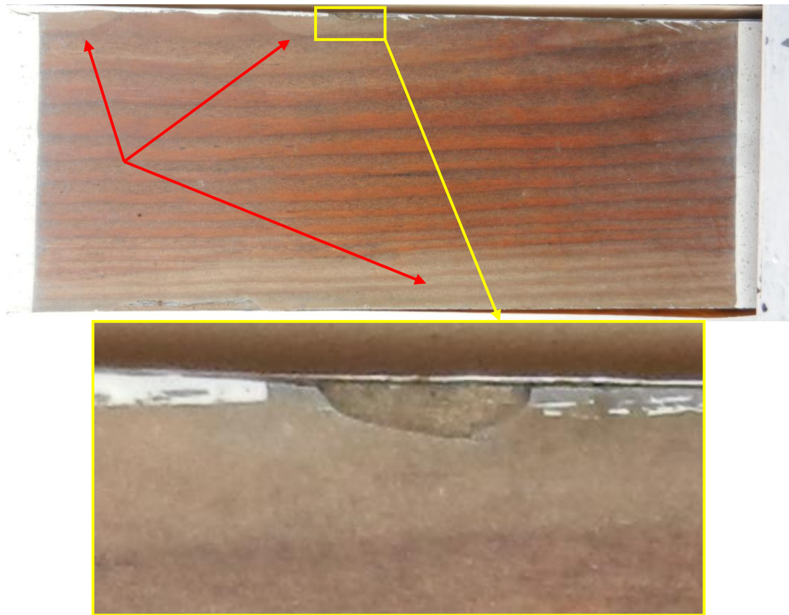
Figure 3: Coating layer delamination occurred to specimen coated with Sayerlack 3 coating system
