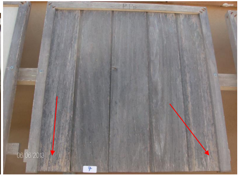
Fig. 11. Cladding 07: XXX Poplar, as in June 2012; (right) The same 07 as in June 2013.
