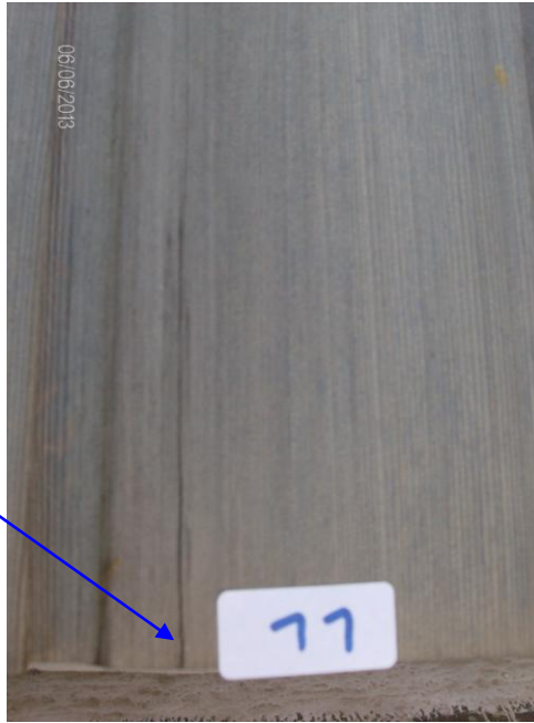
Fig. 26. In cladding no. 11 (Control Western Red Cedar), one small end-splitting was seen.
