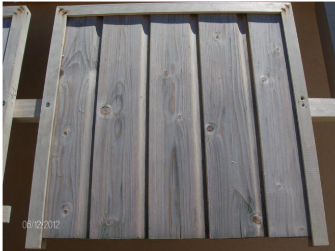
Fig. 14. Cladding 10: Control Spruce, as in June 2012; the same no. 10 as in June 2013
