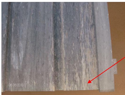
Figs. 27-28. The claddings, no. 07 (XXX Poplar), at left side, and no. 10 (Control Spruce), at right side. In no. 07, an extended weathering appearance and dark & yellow stains. In control no. 10 cladding, the appearance is the worst of all, with lots of defects: cracks, openings, dark stains, extended weathering colour, etc.
