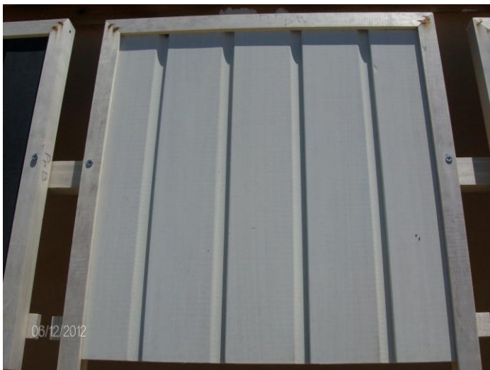
Fig. 8. Cladding 04: XXX Poplar White, as in June 2012; The same 04 as in June 2013 .
