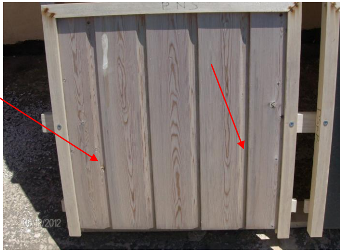
Fig. 7. Cladding 03: XXX Spruce, as in June 2012; The same cladding 03 as in June 2013 .
