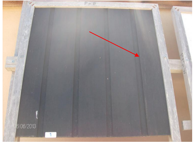
Fig. 5. Cladding 01: XXX Poplar Black, as in June 2012; The same 01 as in June 2013 ; looks good in colour stability.
