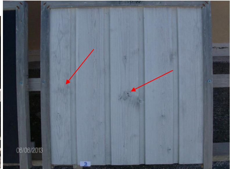
Fig. 13. Cladding 09: XXX Spruce White, as in June 2012; the same no. 09 as in June 2013 .
