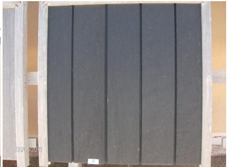
Fig. 12. Cladding 08: XXX Frake Black, as in June 2012; the same (right) no 08 as in June 2013.
