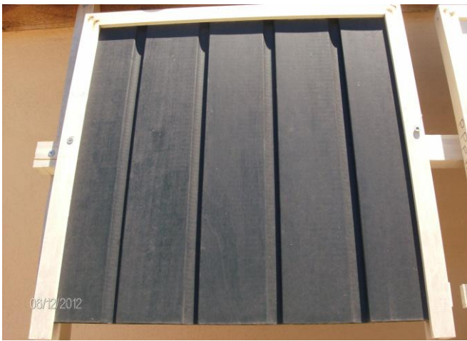
Fig. 5. Cladding 01: XXX Poplar Black, as in June 2012; The same 01 as in June 2013 ; looks good in colour stability.
