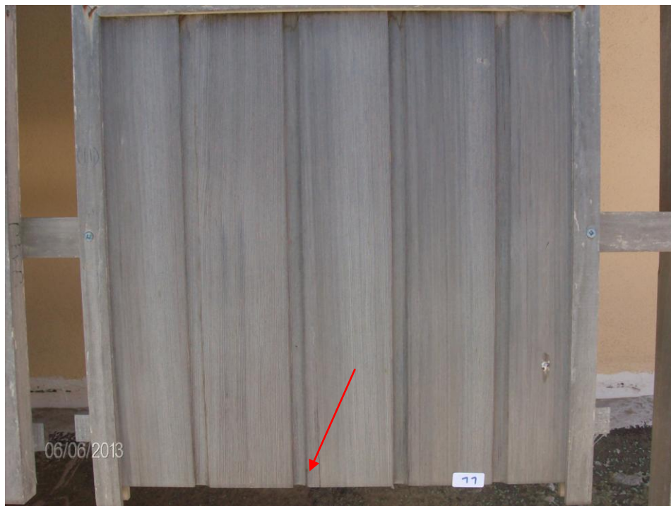
Figs. 15. Cladding 11: Western red cedar (WRC) as in June 2012 (Fig. 15a); (below) The same cladding no. 11, as in June 2013 (Fig. 15b)
