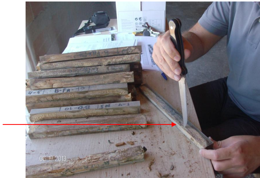
Fig. 32. Application of the “pick-test” as in June 2013 (WFDT, TEI of Thessaly).
