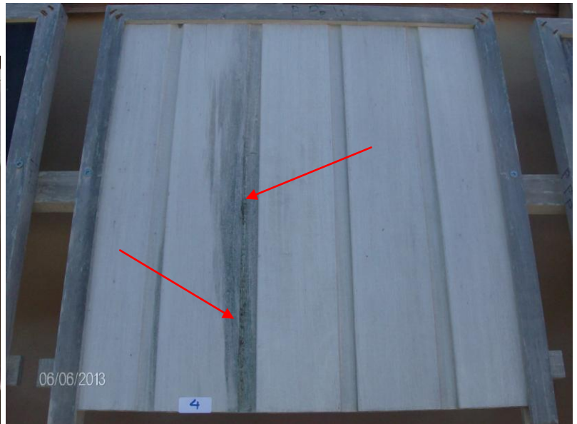
Fig. 8. Cladding 04: XXX Poplar White, as in June 2012; The same 04 as in June 2013 .
