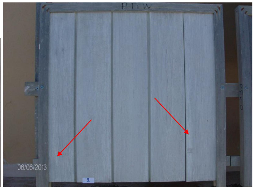
Fig. 6. Cladding 02: XXX Frake White, as in June 2012; The same cladding 02 as in June 2013
