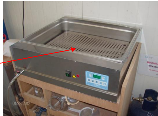
Fig. 16. Modern water bath having a controlled temperature meter.
