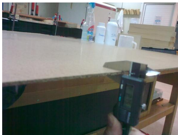
Fig. 8. Measuring the board thickness at the edges
