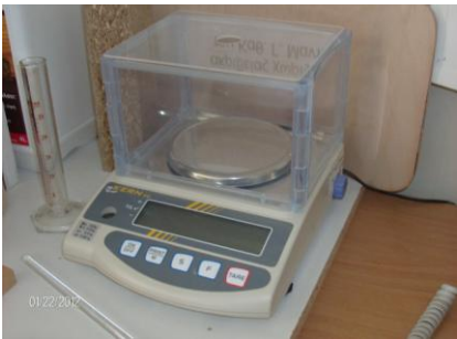
Fig. 4. High accuracy electronic balance with 3-decimals.
