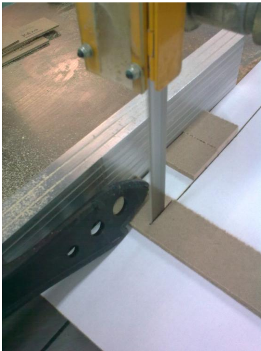
Fig. 2. Cutting of 50mm x 50mm samples for the swelling & absorption tests.
