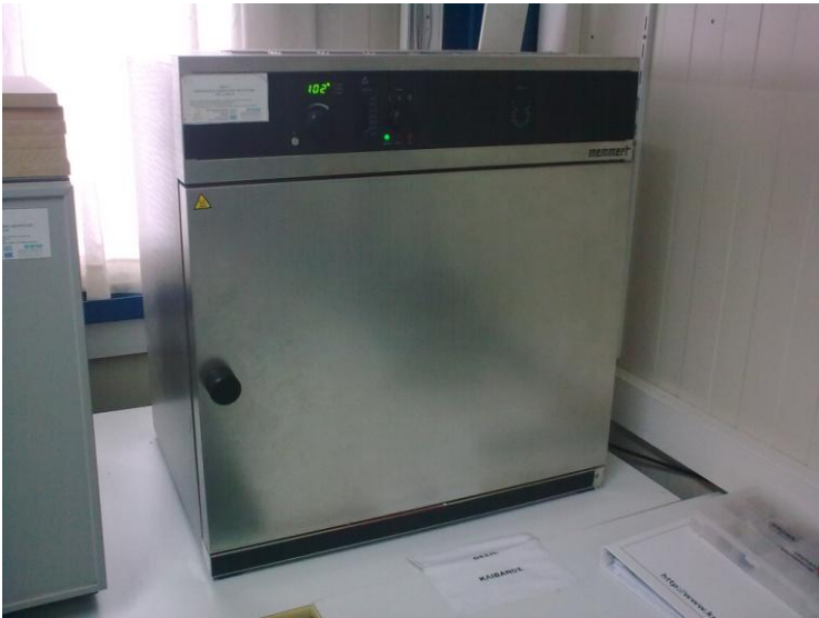
Fig. 5. Drying oven suitable for wood samples with air-circulating system.
