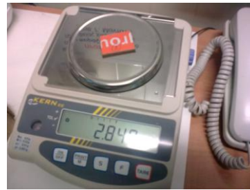
Fig. 6a,b. A hardboard sample (having deformation on a wooden crate) was tested for MC.
