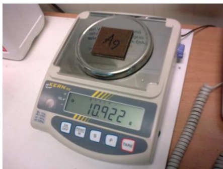
Fig. 17. Weighing wet specimens
