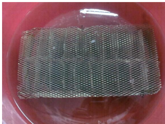
Fig. 18. Metal basket used for absorption tests.
