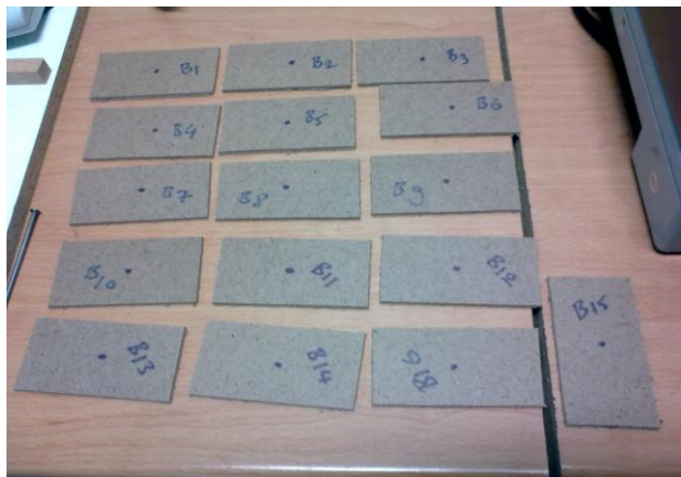
Fig. 3. Specimens cut for the bending strength MOR tests (measuring 95mm x 50mm).
